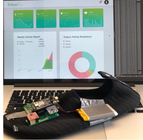
Fig. 6. FitFeet Shoe on a printed circuit board with attached battery, IMU, and Haptic controller attached
