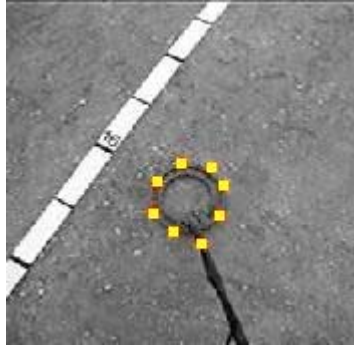
Fig.3. Metal detector head tracking result. The square dots indicate the tracked target
